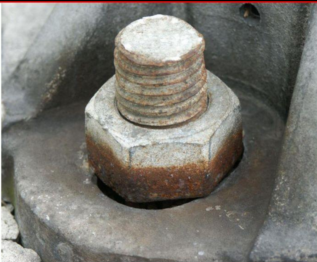
Galvanized bolting assembly after ten years of exposure to a deicing salt environment.
